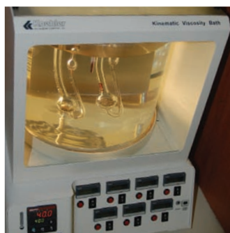
On site Viscosity testing
